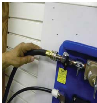
9. Attach water inlet. Make sure that strainer washer provided is installed.
