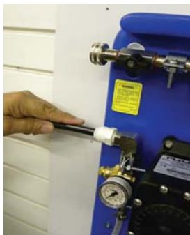
8. Attach air inlet tubing. Use reducers as needed.
