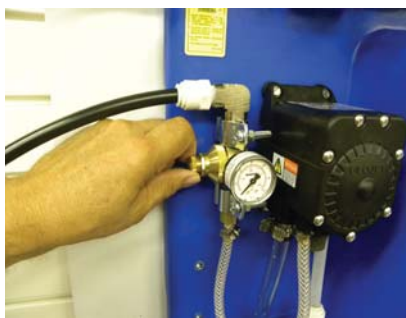
11. Adjust the air pressure as desired (100 PSI max, 20 PSI minimum).
